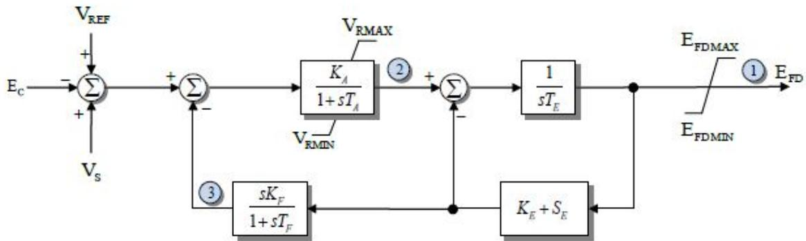
Figure 3: IEEE1A Block Diagram [5]
